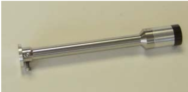
Figure 11 Geometry holder for use without the upper fixture.
