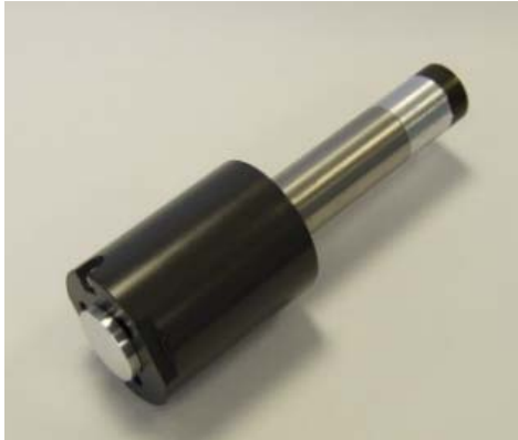
Figure 10 Geometry holder for use with the upper fixture.
