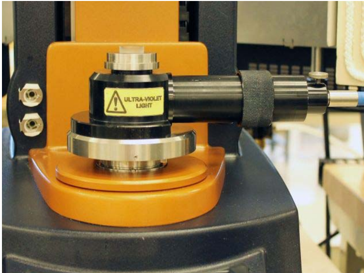
Figure 9 Fully installed light guide lower fixture.
