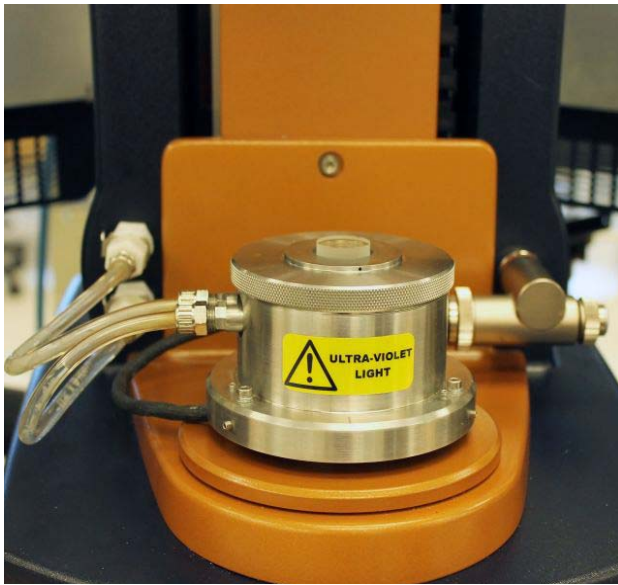
Figure 5 LED lower fixture mounted on the rheometer.
